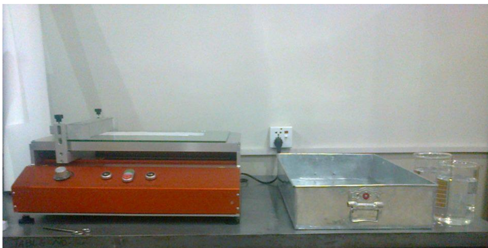
Figure 3.1: Thin film applicator used for membrane casting.
