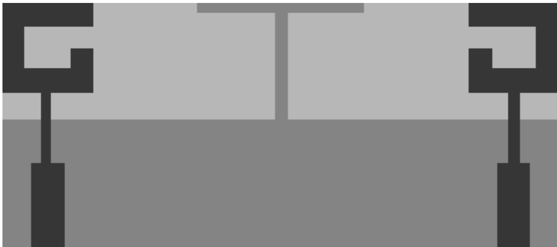
Figure 2.13 Structure of G-shaped MIMO [31]
