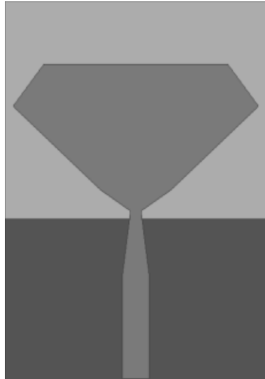
Figure 2.10 Diamond Shaped UWB antenna [28]
