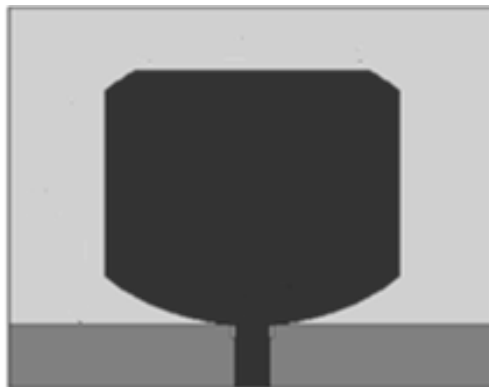
Figure 2.2 UWB Antenna with round junction [18]
