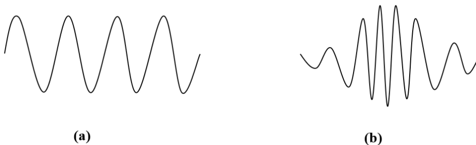
Figure 3.3 Comparison (a) sine wave (b) wavelet
