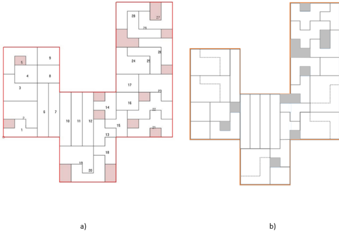
Figure 5.5: Experiment 2: a) Doraid Dalalah [3] with sheet utilization of 89.7% b) Proposed approach with sheet utilization of 93%
