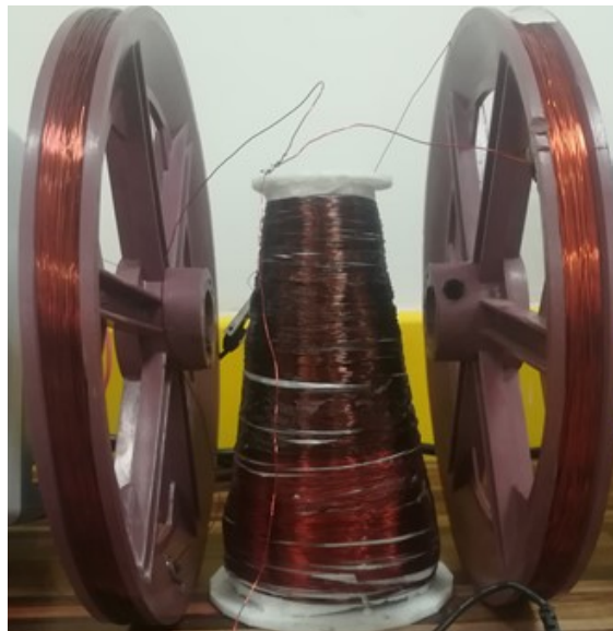
Figure 5.4: Helmholtz Coil with Cone-Coil in middle
