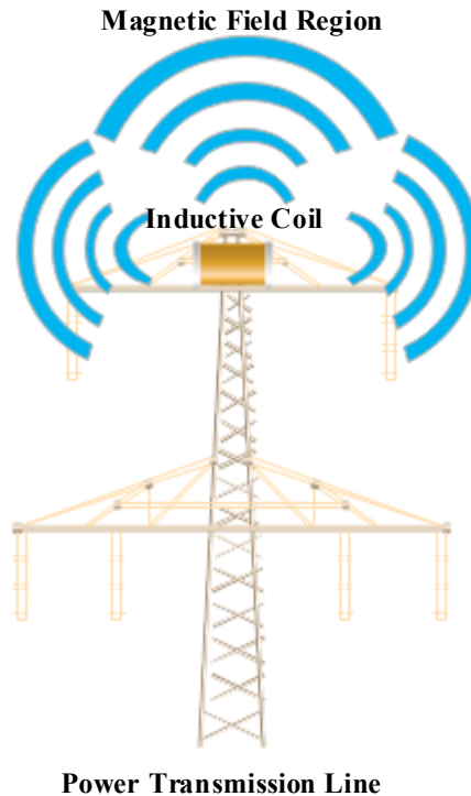
Fig 1.5: Model Diagram of Energy Harvesting by Inductive Coupling method from Power Lines
