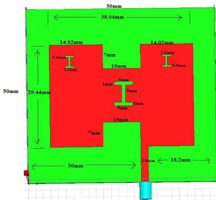
Figure 2.13 H shape microstrip fed off centre
