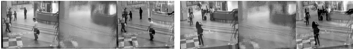
Figure 4.4: Airport sequence : Using subsampling (Subsampling rate =0.01) From left to right, Original Frame, Extracted Background, Foreground (Residuals).
