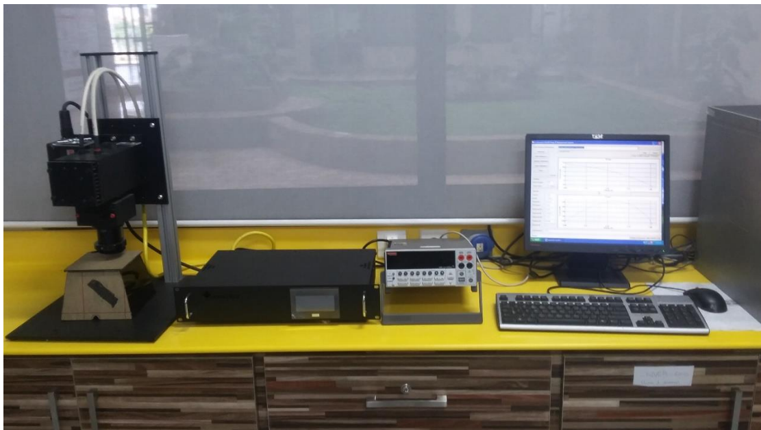
Figure 3.4 Solar Simulator available at USPCASE, NUST
