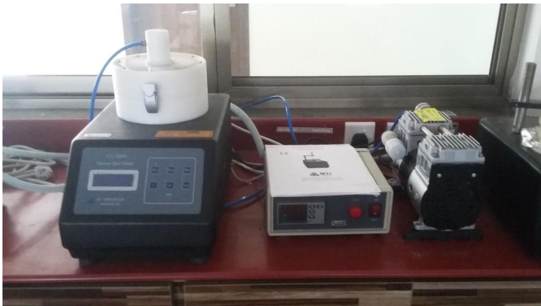
Figure 3.1 Spin Coater available at USPCASE, NUST for deposition of various layers
