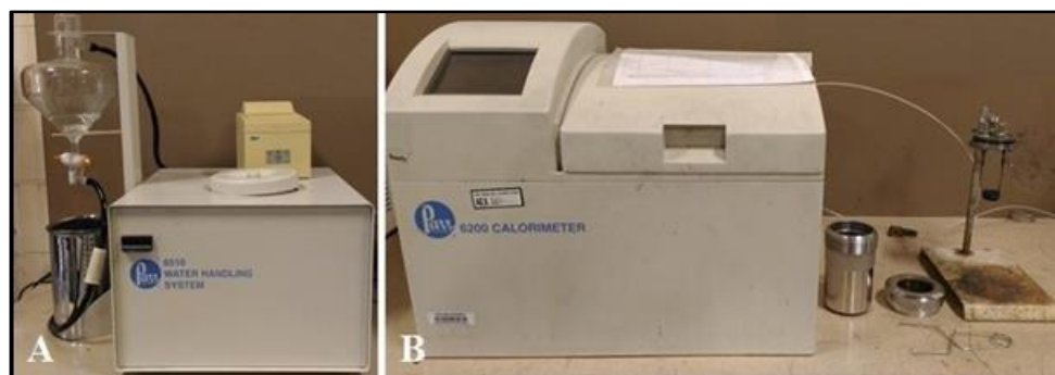
Figure S 6 6200 Isoperibol Bomb Calorimeter
