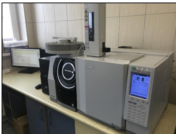
Figure S 7 Shimadzu gas chromatograph-mass spectrometer GCMS-QP2020 NX
