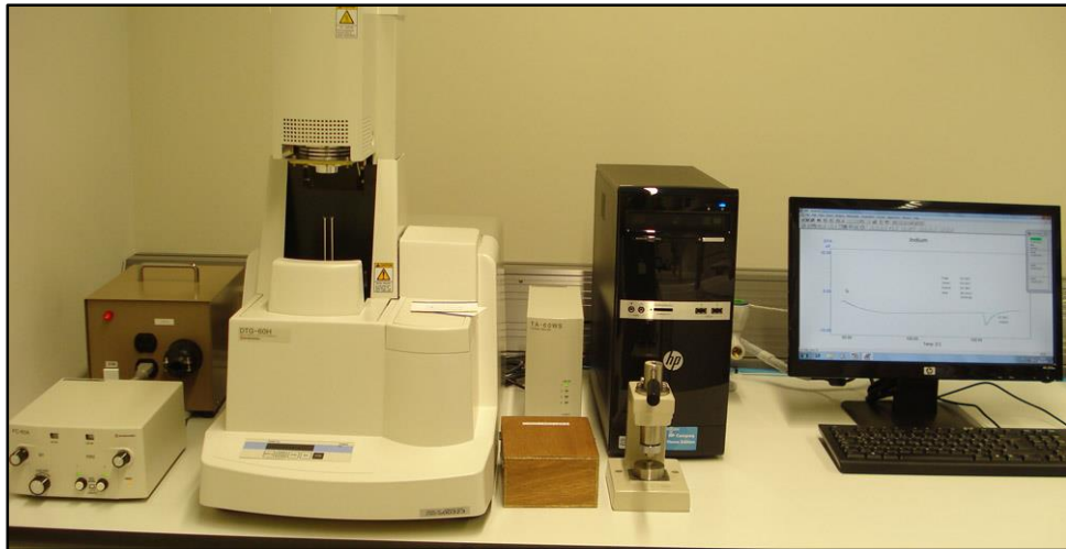
Figure S 3 SHIMADZU-DTG 60H Thermo gravimetric instrument
