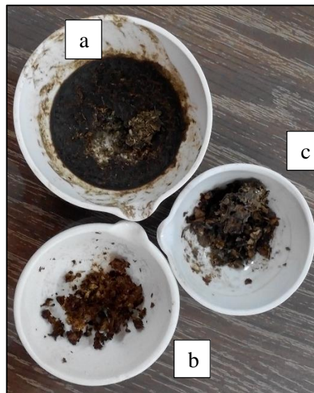
Figure 3.4: Samples inoculum (a), cabbage (b) and potato (c) after drying at 105 o C in the drying oven.
