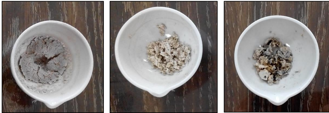
Figure 3.5: Samples inoculum (left), cabbage (centre) and potato (right) after ignition at 550°C in the muffle furnace.
