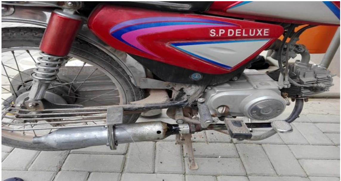
Figure 10: Catalytic converter mounted on motorcycle's exhaust for final testing
