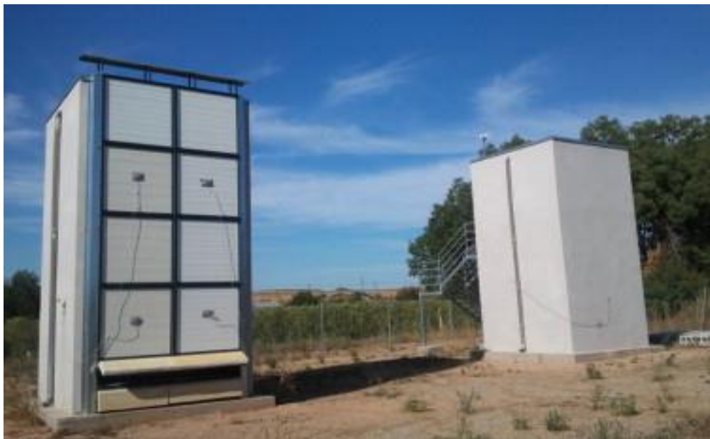
Figure 2.6: Ventilated Façade with PCM cold storage [14]
