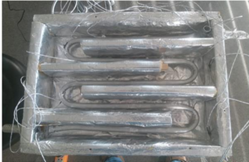
Figure 4.7: Channels for air passage
