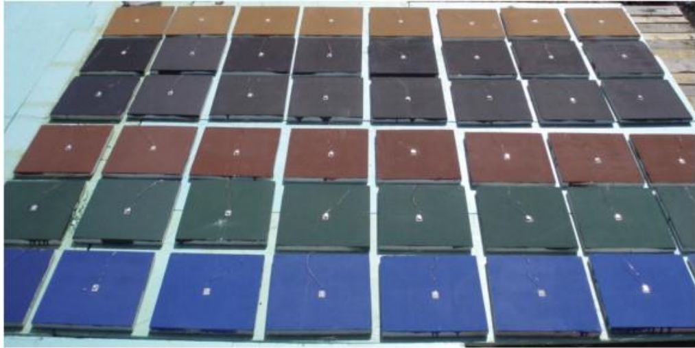
Figure 2.3: Testing tiles coated with PCM [6]
