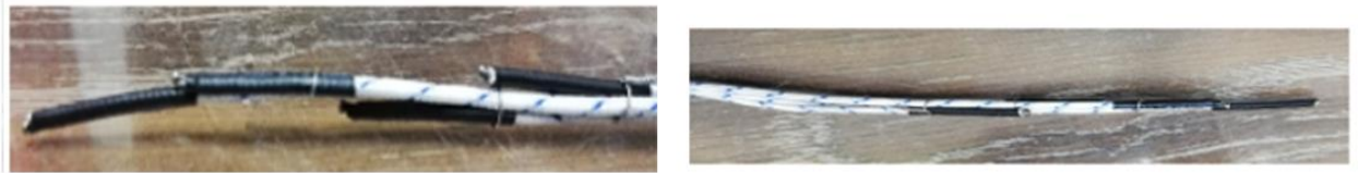
Fig. 4-8: Thermocouples stacked for monitoring the inside temperature of the cylinder (centerline)
