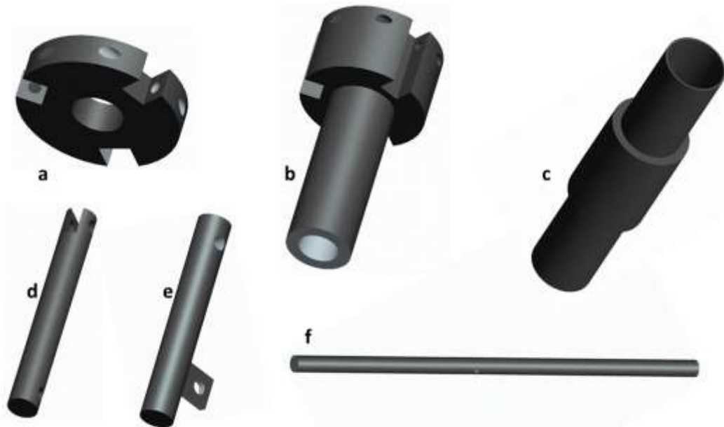
Figure 3.1: Illustrating different parts of the device, (a) Cylindrical part fixed with main rod having pin joints with spokes, (b) Cylindrical moving parts which slides over both the sides of rod having pin joints with spokes, (c) Cylindrical moving parts which slides over both the sides of rod having pin joints with spokes, (d) Rod with pin joint, (e) Rod with pin joint, (f) Main rod.
