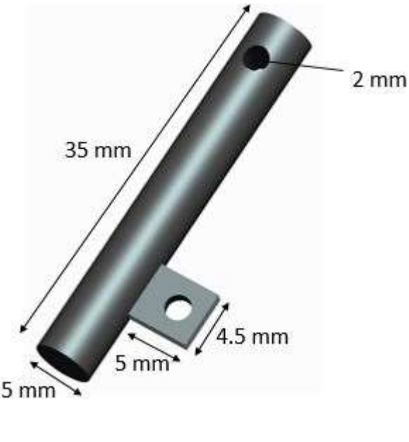
Figure 3.2: In-silico design and Measurements of (a) main rod (b) hollow cylinder (c) sliding part
