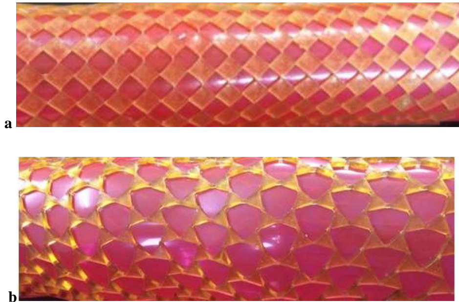
Figure 3.13: (a) Rotating square geometry auxetic stent mounted on balloon, (b) Rotating triangle geometry auxetic stent mounted on balloon.
