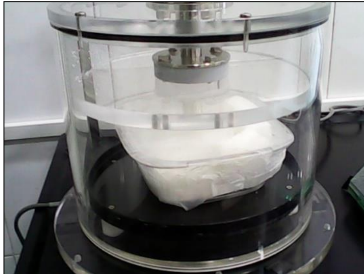
Figure 20: Chitosan-Gelatin sponge mixture kept in freeze dryer
