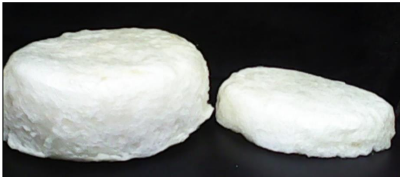
Figure 22: Left) Chitosan-Gelatin sponge crosslinked with 5% Glutaraldehyde 0.1 ml/100 \mu l dissolved whipped mixture (Right) Chitosan Gelatin sponge crosslinked with 0.05ml/50 \mu l of Glutaraldehyde dissolved in whipped mixture.
