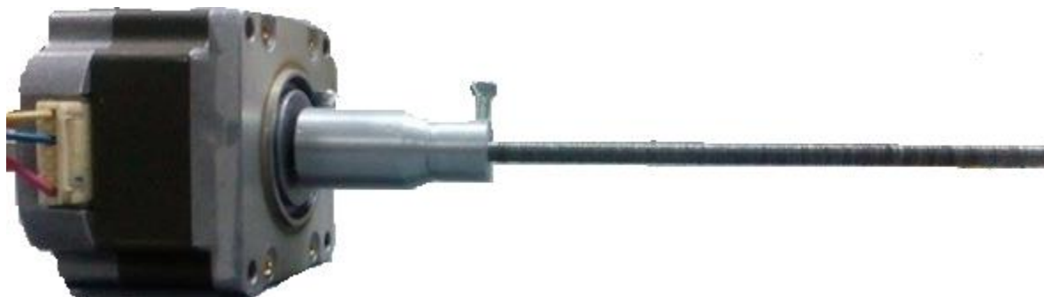
Figure 10: M6 threaded rod coupled to shaft of stepper motor through aluminum coupling
