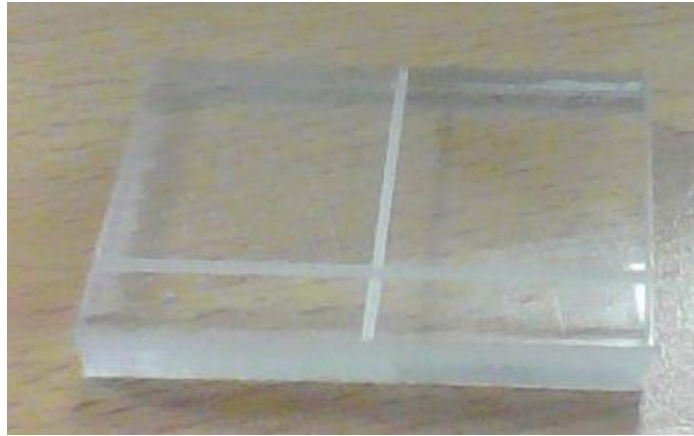
Figure15: channels fabricated on acrylic slab
