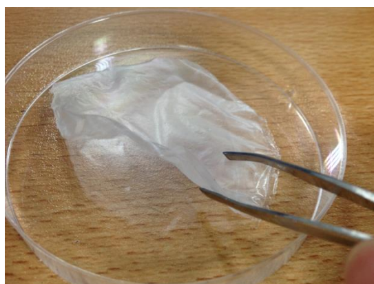
Figure 5: Erythromycin loaded spin coated PVA/PLA ultra-thin polymer film.
