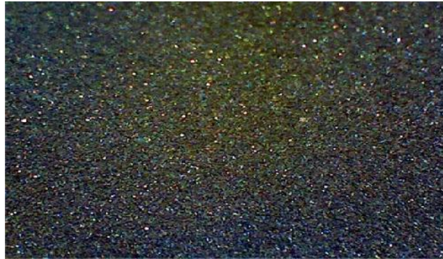
Figure 6 Unsintered copper printed film Optical microscope image at 40X
