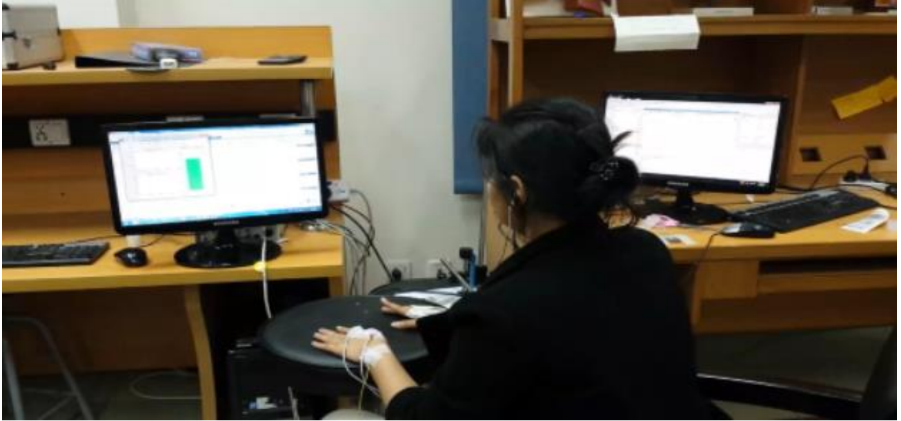
Figure 18: Experimental set-up for the real-time single trial phase synchrony detection of EMG signals.
