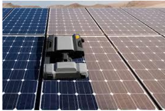
Fig. 2-16: Automatic wiper based cleaning [31]
