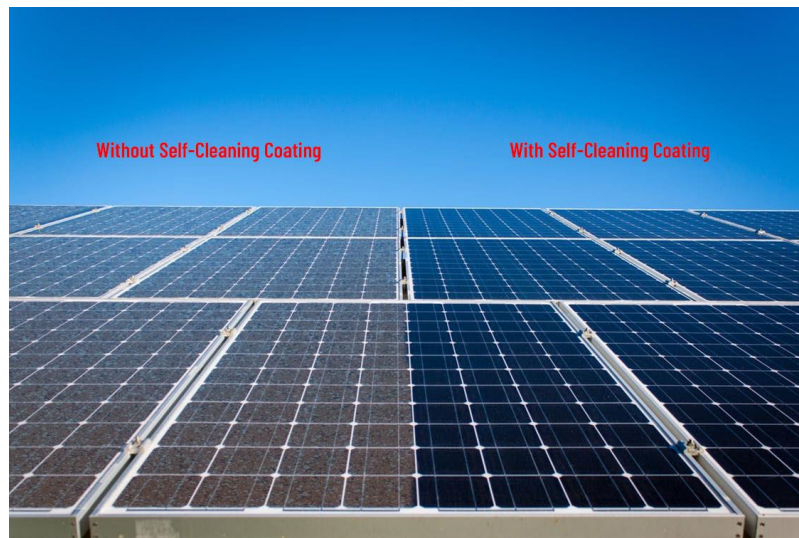
Fig. 2-21: Super Hydrophobic Antireflection coating PV modules [37]
