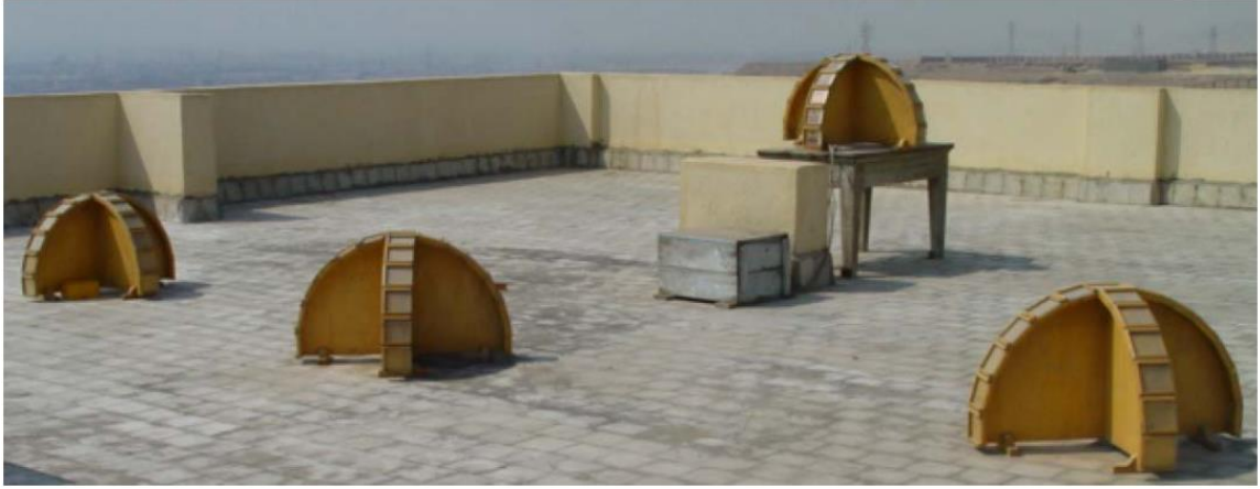
Fig. 2-13: Glass samples exposed to the environment for dust collection [15]
