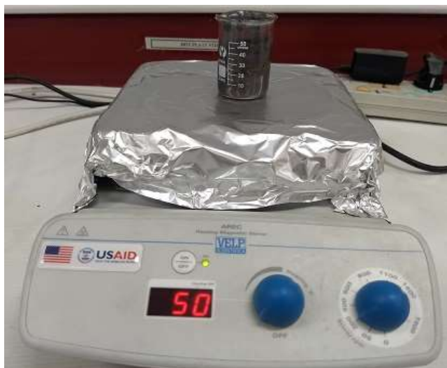
Figure 39: Silicon slurry preparation
