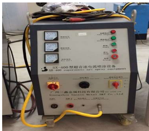
Figure 37: Wire Arc spray System
