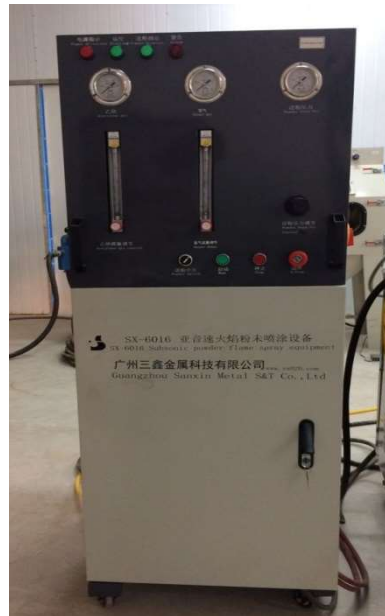
Figure 40: Powder Spray system for top coat deposition
