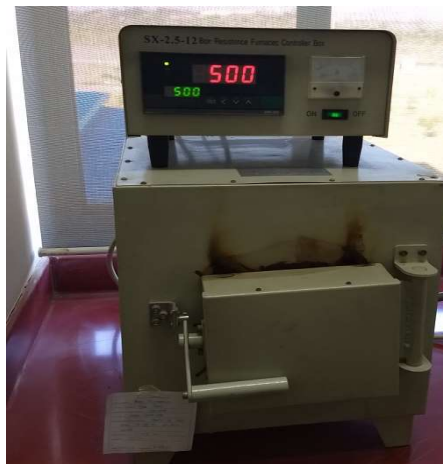
Figure 38: Nickel-Aluminide formation via thermal annealing
