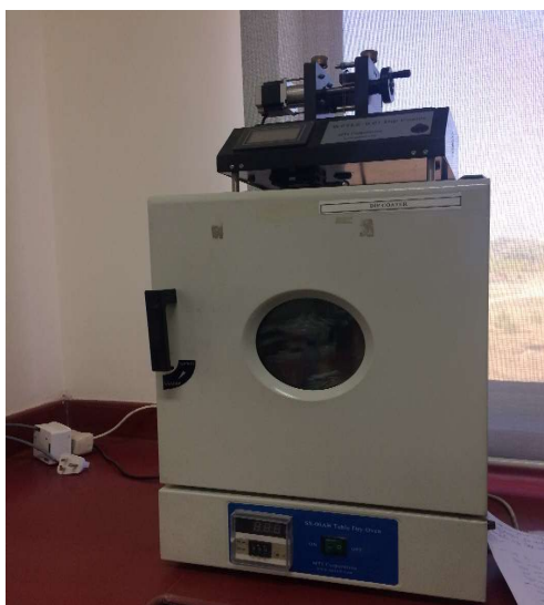
Figure 23: Dip Coater equipment used in AEMS Lab.
