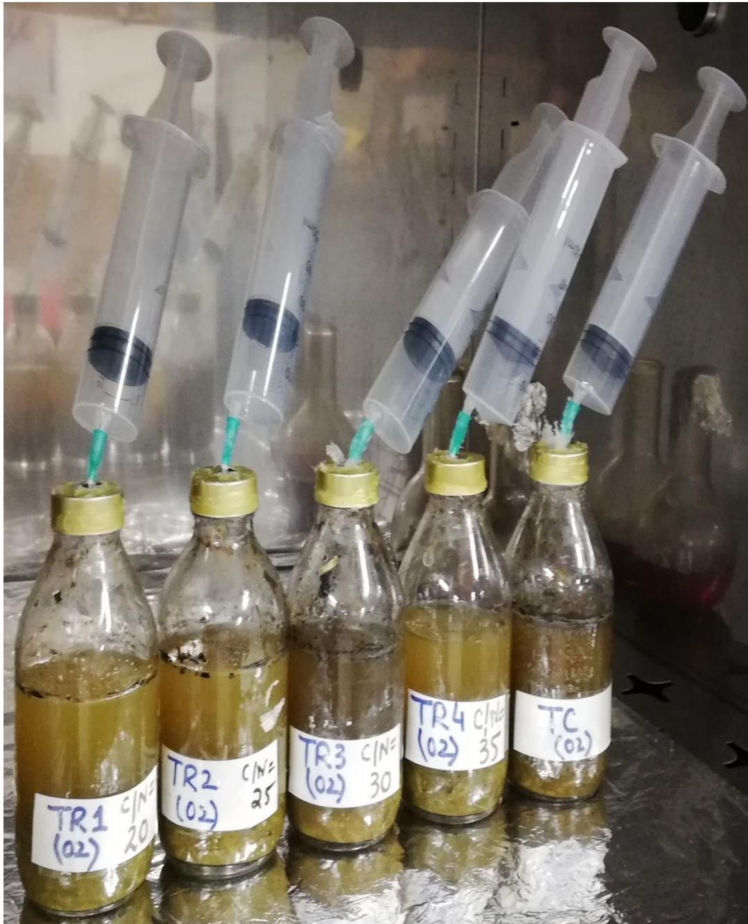
Figure 3.6: Lab scale batch type reactors setup at thermophilic temperature.
