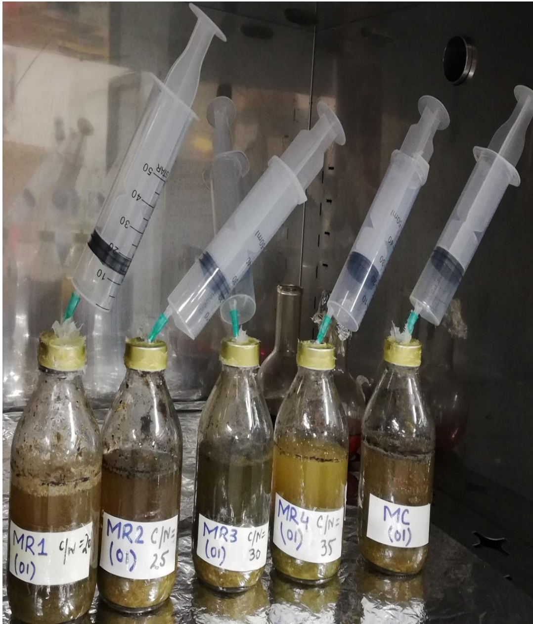
Figure 3.5: Lab scale batch type reactors setup at mesophilic temperature.
