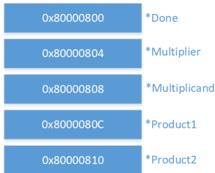
Figure 8.17: Address Pointer Declaration for Variables (32-bit)
