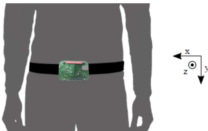
Figure 3.1 Waist mounted custom made embedded device used for data acquisition comprising of a gyroscope and two accelerometers
