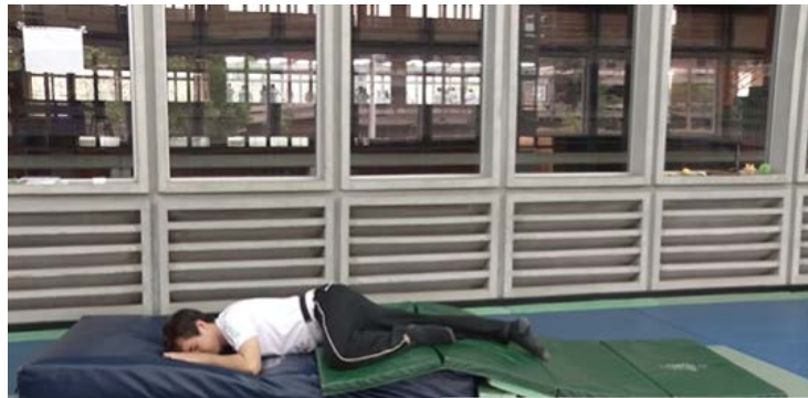
Figure 3.2 Fall F01: Forward fall when walking triggered by a slip performed by a subject
