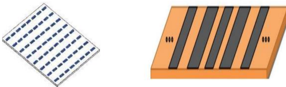
Figure 2.22: (a) Short dipole type FSS surface (b) Long strips type FSS surface
