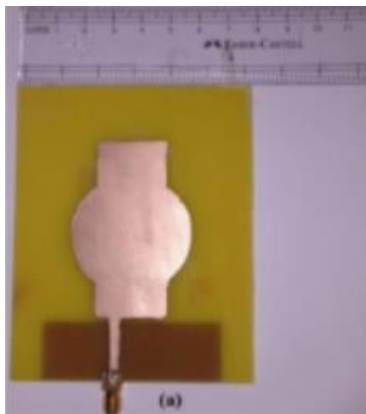
Figure 2.6: UWB Antenna with both circular and rectangle shape
