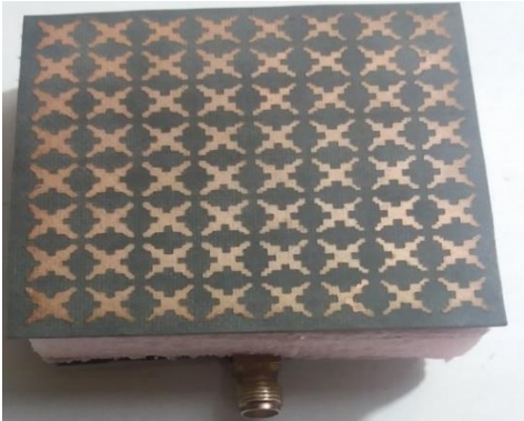
Figure 4.5 Antenna with FSS at a separation distance of 4 mm
