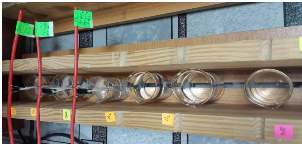
Figure 3.2: Layer by Layer assembly setup for coating on fabric.
