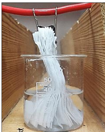
Figure 3.1: Pre-treatment of fabric with APTMS aqueous solution
