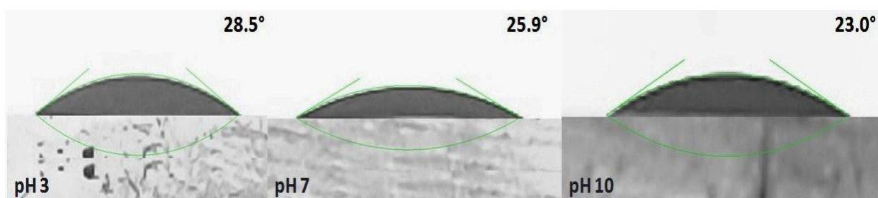
Figure 4.10: Contact angle images of samples with PDADMAC as the top layer.
