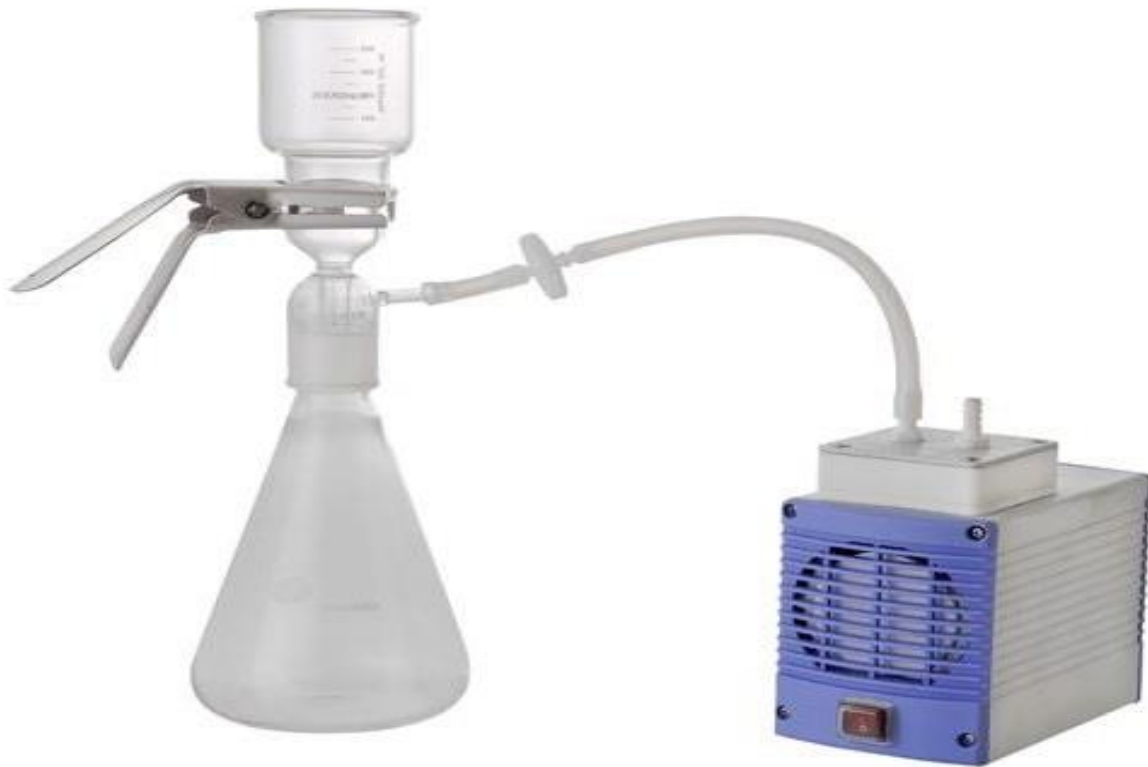
Figure 10: The filtration equipment used to test the permeation performance of the prepared membranes.
