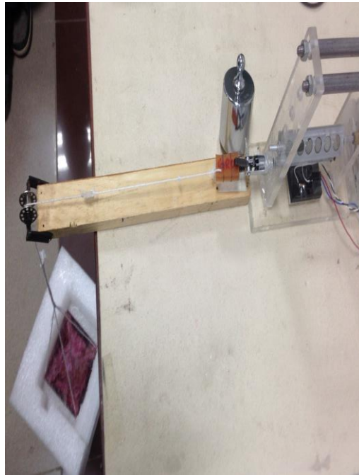
Figure 29. Vertical Slippage Test Setup
