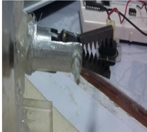
Figure 34. Sensor held between the grasper teeth
