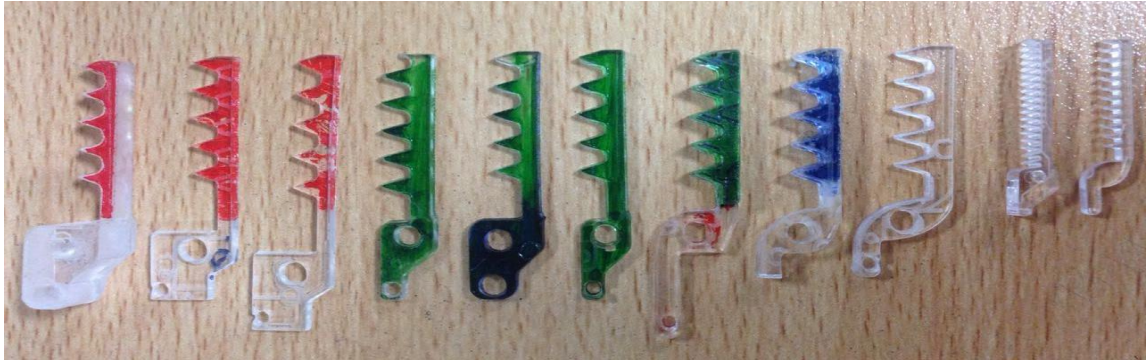
Figure 7. Grasper various designs fabricated using Laser machine
