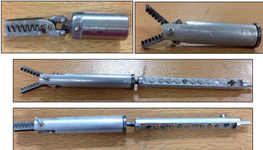
Figure 19. (a) Assembled Grasper with the lead head, (b) Assembled grasper with the outer aluminum pipe, (c) Opened Grasper with the magnetic array, (d) Closed Grasper with the magnetic array
