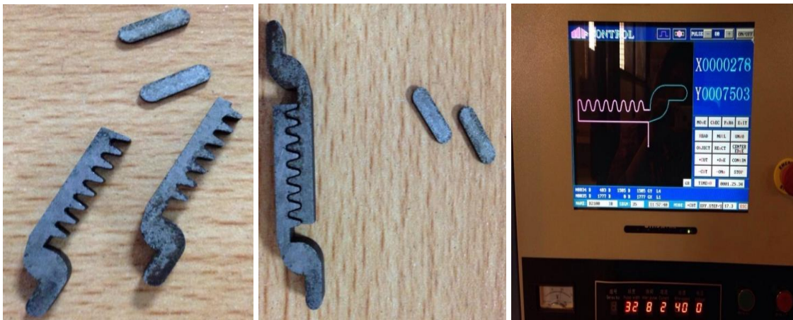
Figure 10. Illustrating different parts of the prototype fabricated using EDM Wire Cut Machine, (a) &(b) Grasper Jaws and short bars, (c) CNC EDM Wire Cut machine cutting the CAD design of grasper jaws
