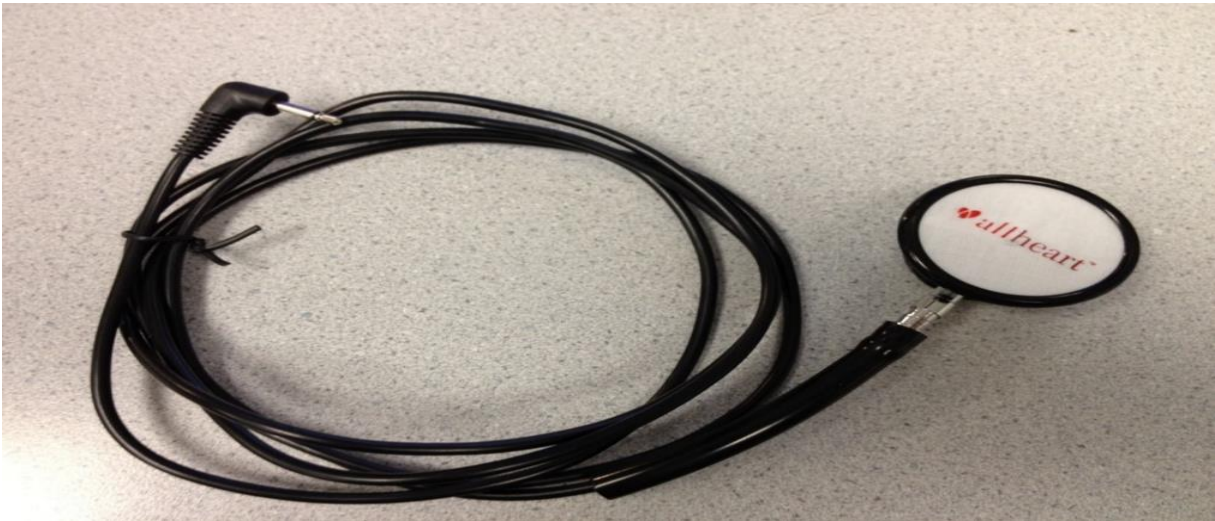
Figure 2.2. Assembly of High Sensitive Microphone Attached with Chest-piece
