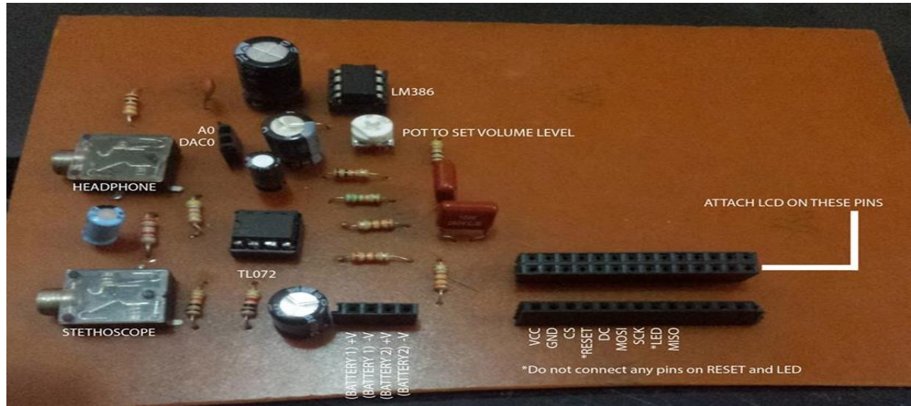
Figure 3.2. Hardware Implementation of Circuit on PCB Sheet
