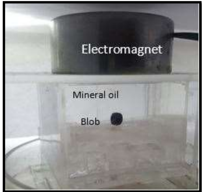
Figure 9: Main setup used for navigation, electromagnet provides driving force to drive the blob in mineral oil.
