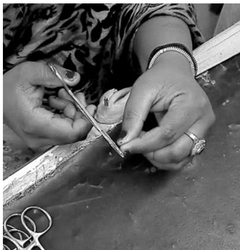
Figure 5: Needle Holder Thread Tension Testing by hand
