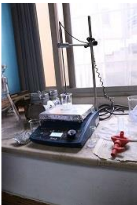
Figure 7: Image showing experimental set up on a digital magnetic stirrer
