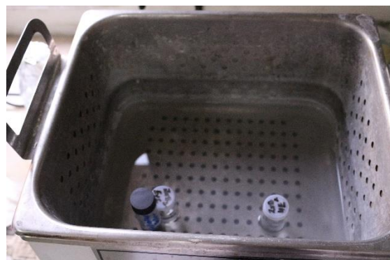
Figure 8: Image showing experimental set up of mixing organic phase in a Sonicator
