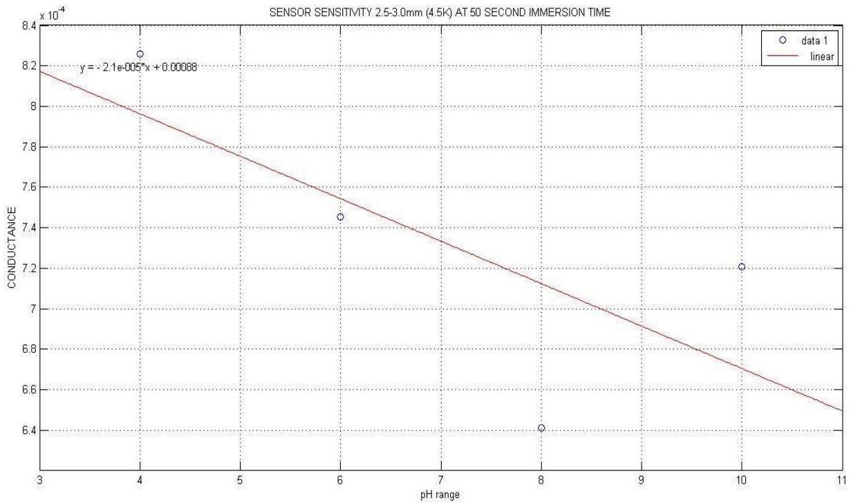
Figure 4.8 pH-Conductance box plot for pH 4,6,8,10;Sensor sensitivity for the size 2.5-3.0mm
