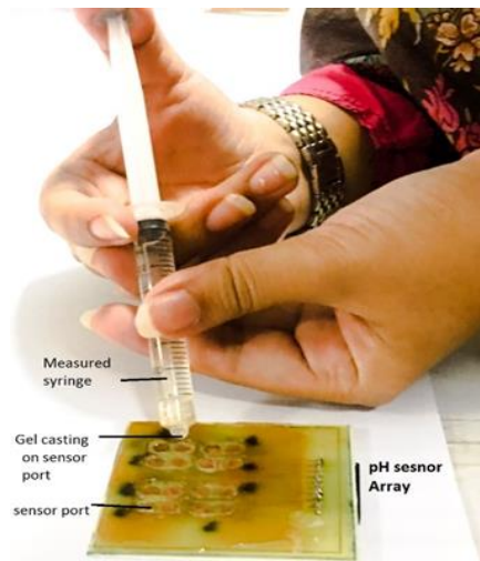
Figure 3. 6. Shows casting of hydrogel on conductive sensor port of pH sensor array
