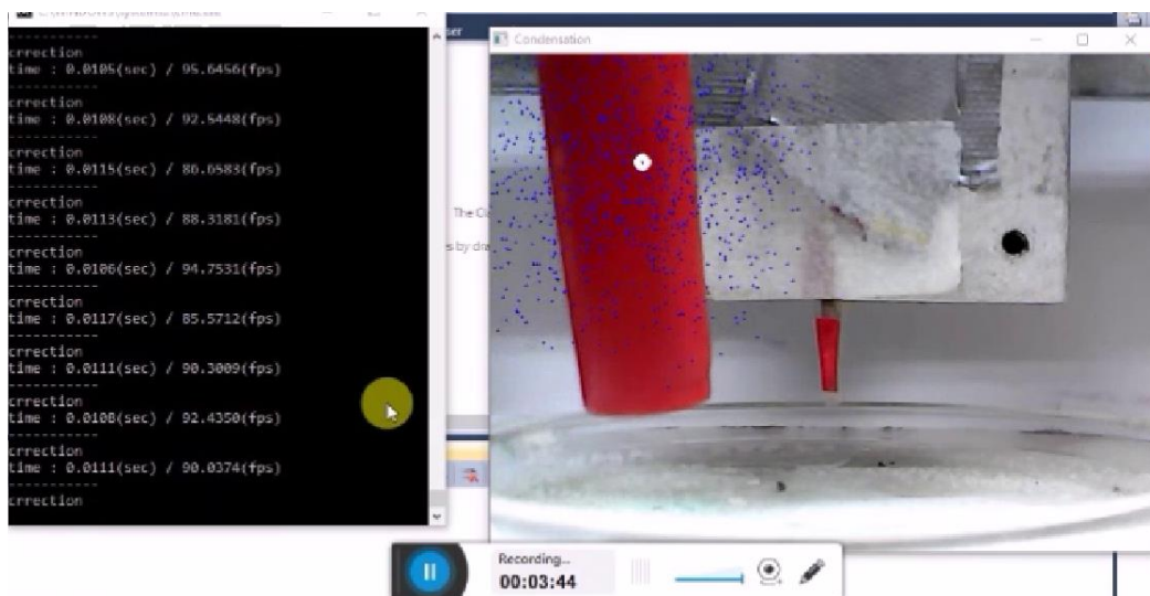
Figure 45: Red Particle Filter results. It prefers higher saturation
