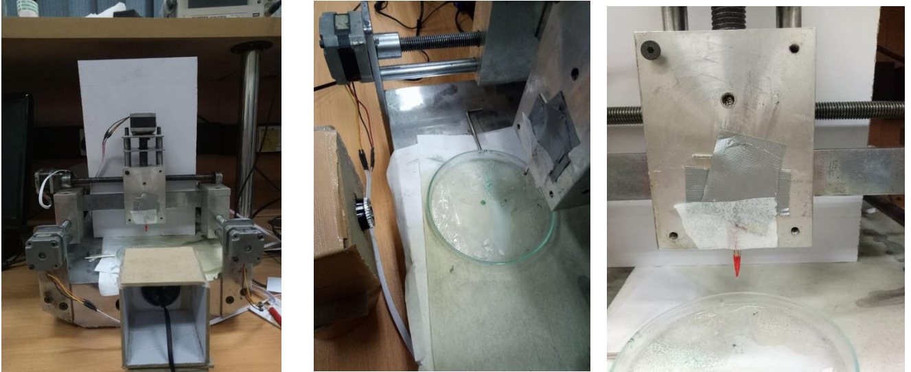
Figure 6: Vision acquisition setup with XYZ lead screw stage used for linear motion along z axis
