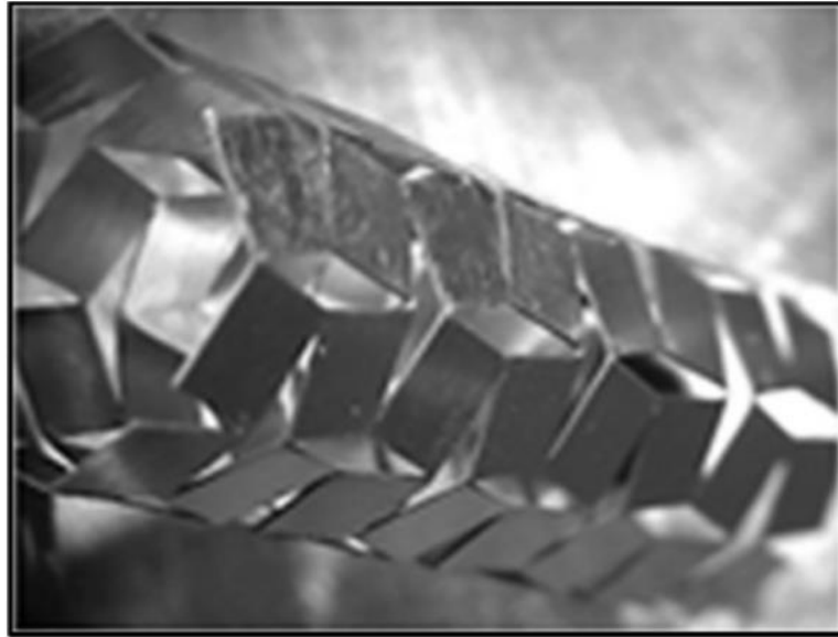
Figure 2. 10: Drug delivering auxetic stent (Bhullar et al. , 2015).
