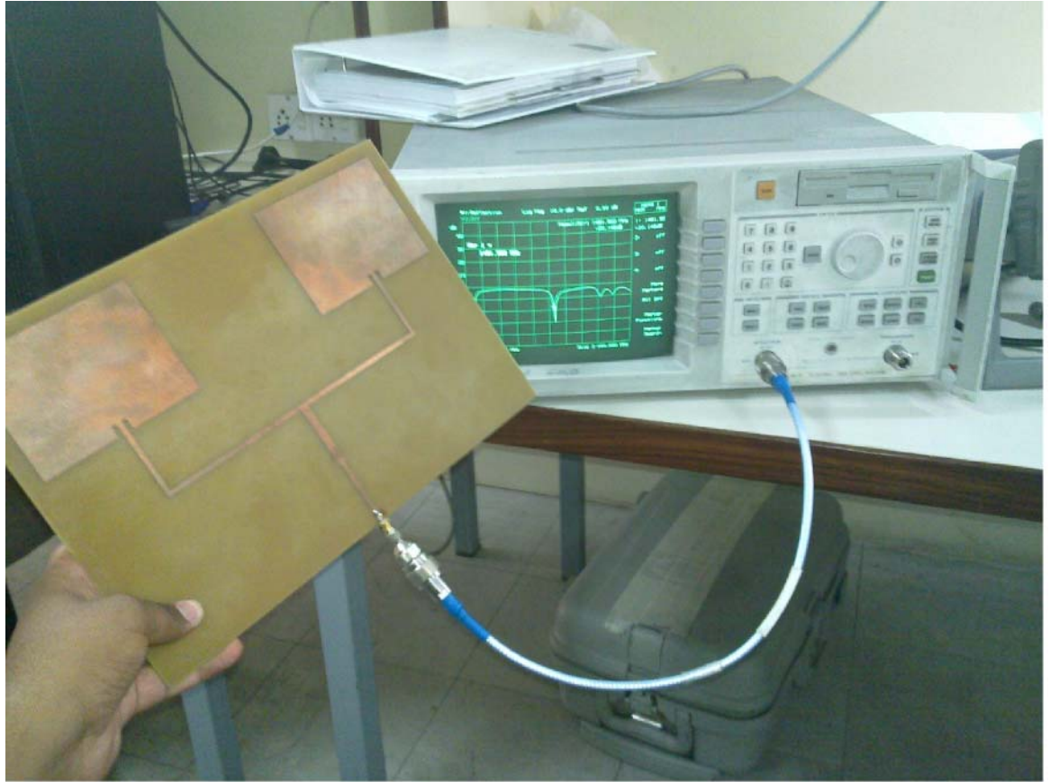
Figure 7.2 FR4 Test Antenna resonating at 944.4 MHz
