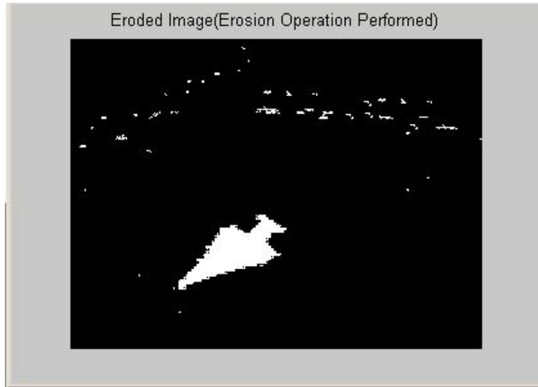
Figure 9 Erosion Operation Performed on Binary Image
