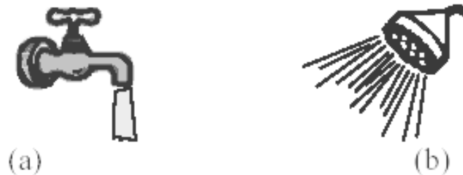
Fig-4.3 a) A regular FDM signal with all data on a single big data stream. b) An OFDM signal with multiple parallel bit streams carrying same amount of data.
