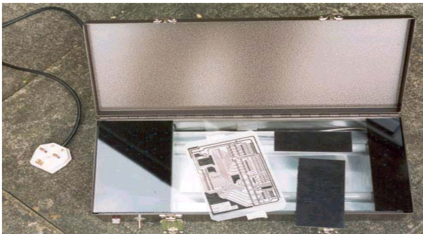
FIGURE 6.3 Light box being used for exposing [13]
