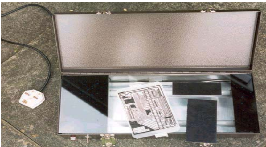
FIGURE 6.3 Light box being used for exposing [13]
