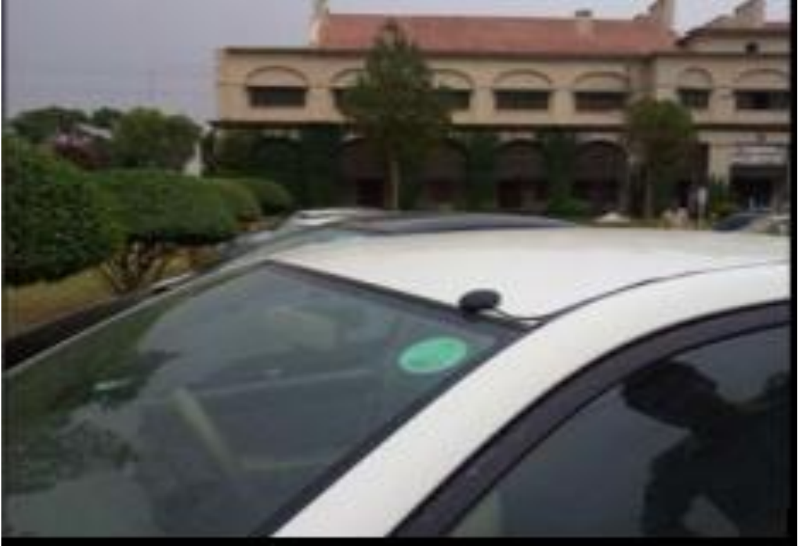
Figure 6.1 Installation of GPS dongle
