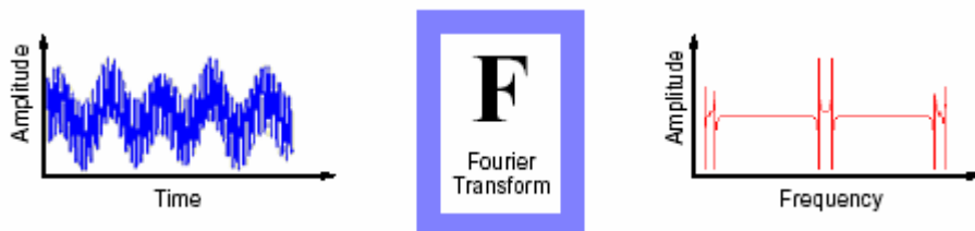
Fig 8: Fourier transform of a time domain signal
