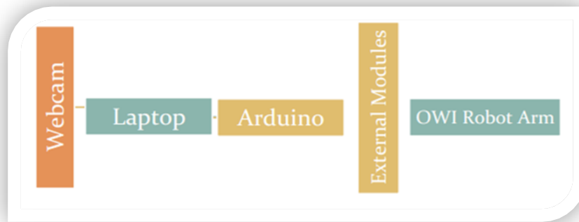
Figure 1: Block Overview of the Designed System
