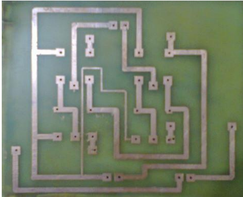
Figure 19 : Motor Driver pcb design
