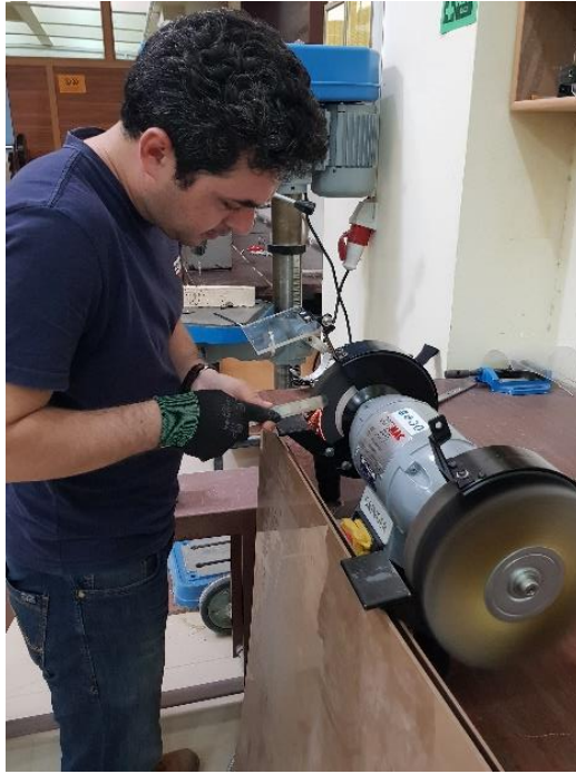
Figure 16 Grinding of mechanical parts to acquire shape
