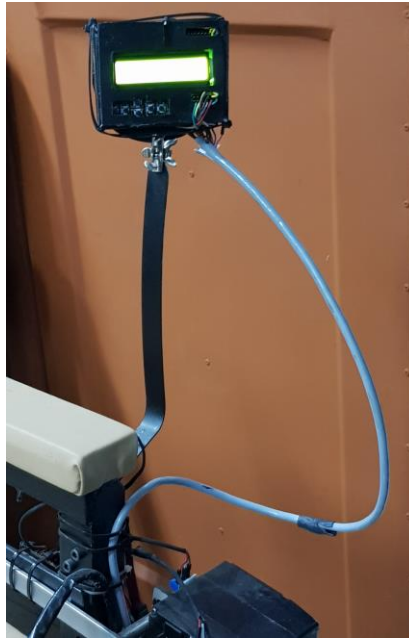
Figure 28 Controller with display mounted on a bar adjacent to device
