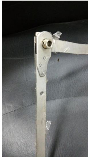
Figure 19 Titanium joint modification for motor attachment
