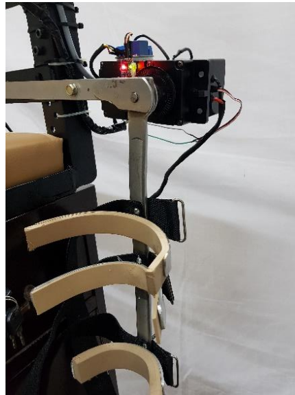
Figure 20 Joint modification for securing leg
