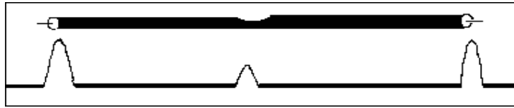
Figure 4-2 Amplitudes of the reflections due to impedance change [10]
