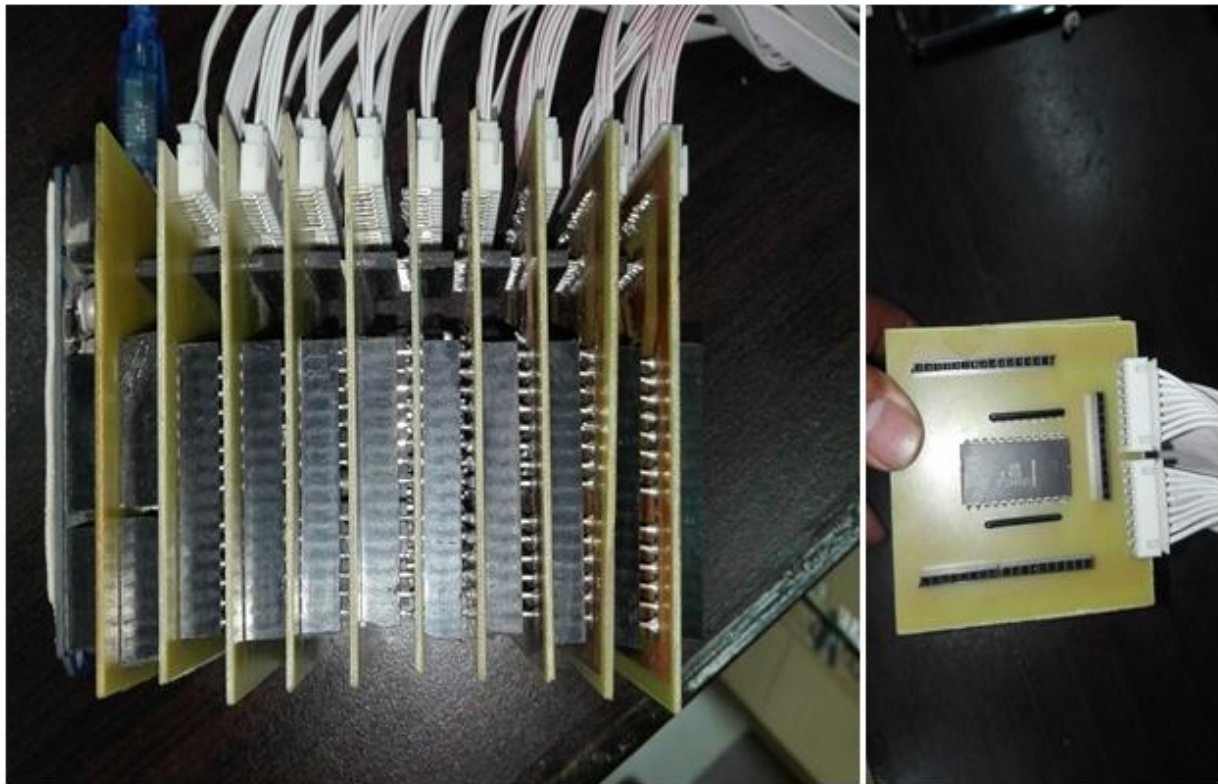
Figure 5 Arduino, Selector Board and Mux Boards in Order from Left to Right
