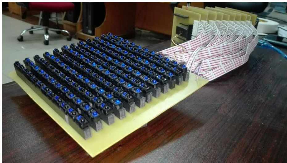
Figure 7 Final Sensor Board and Mux Boards Connected
