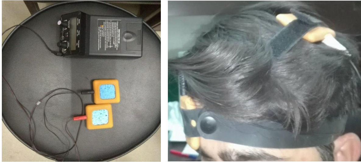
Figure 11 tDCS Device with sponge electrodes (left), Subject with Electrodes Attached at C3 and FP2
