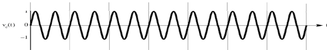
Carrier signal \cos \omega_c t
