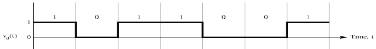
Binary Modulating Signal m(t)
