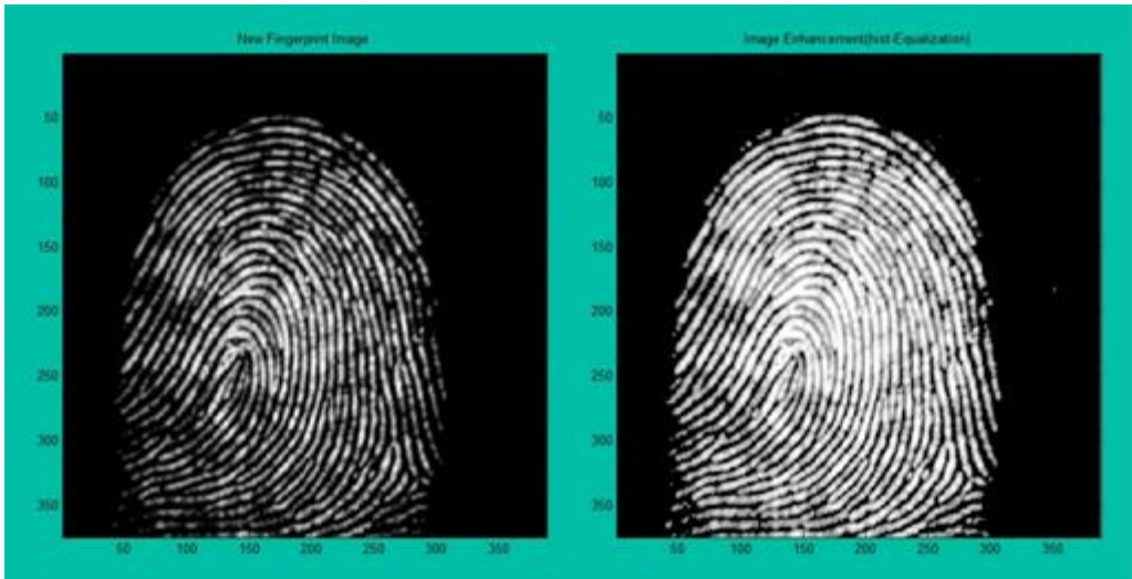
Figure 5.3 Histogram Enhancement. Original Image (Left). Enhanced image (Right)
