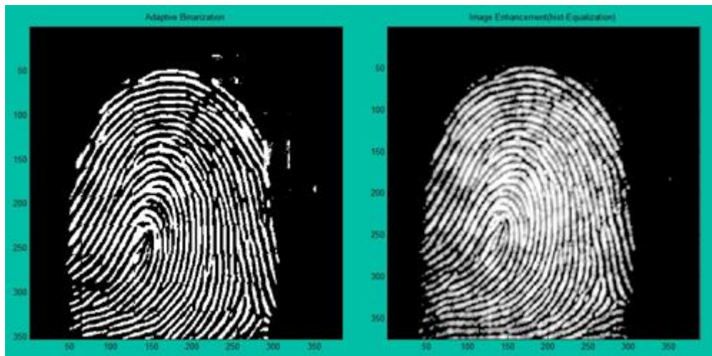
Figure 6.1 the Fingerprint image after adaptive binarization Binarized image (left), Enhanced gray image (right)
