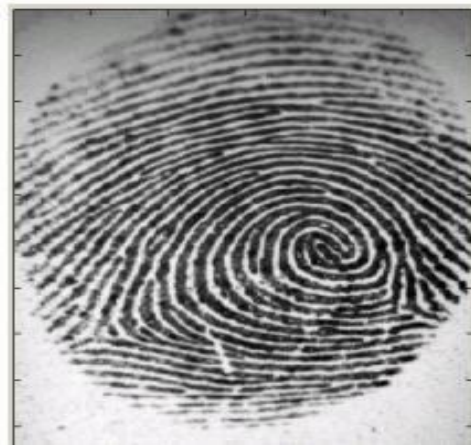
Figure2.1 A fingerprint image acquired by an Optical Sensor
